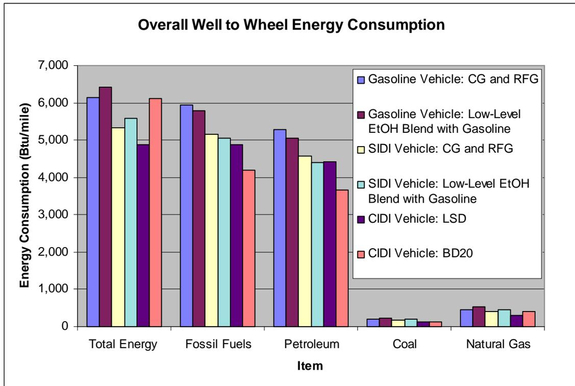
Figure 3.4.16 WTW energy consumptions for competing vehicle-fuel combinations
