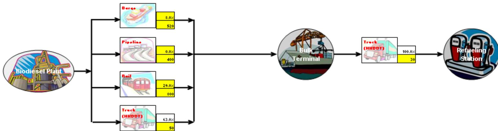
Figure 3.4.6 Transportation & distribution process diagram for biodiesel
