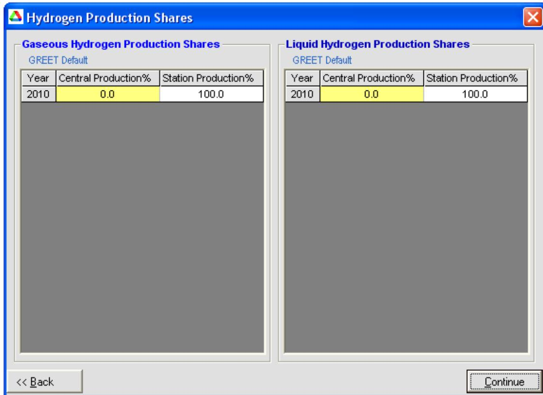
Figure 2.4.14 The hydrogen production shares window contains the yearly market share information for central and station production. <sup>[4]</sup>
