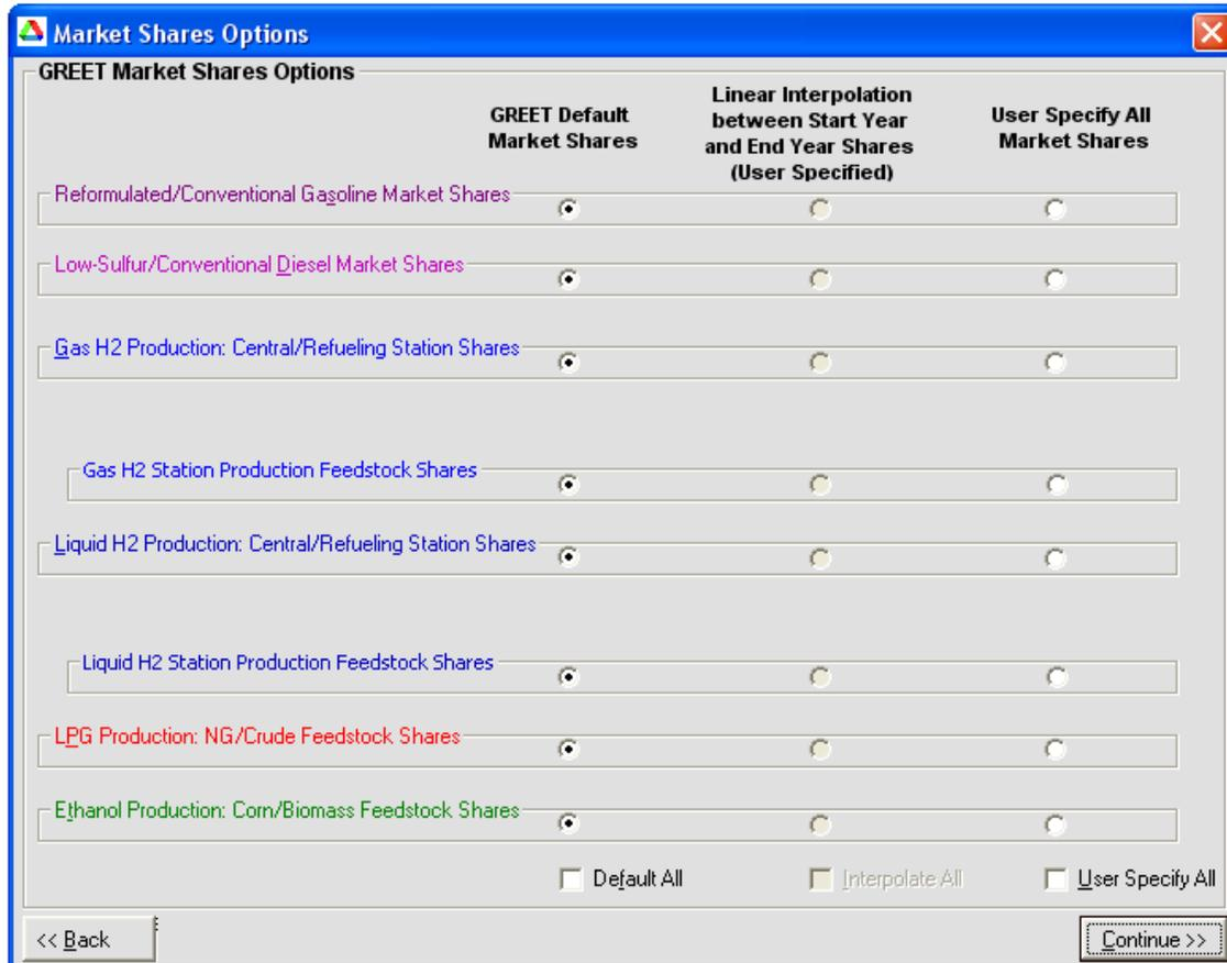
Figure 2.4.12 The market shares options window allows the method for determining market shares to be specified for individual markets. <sup>[4]</sup>
