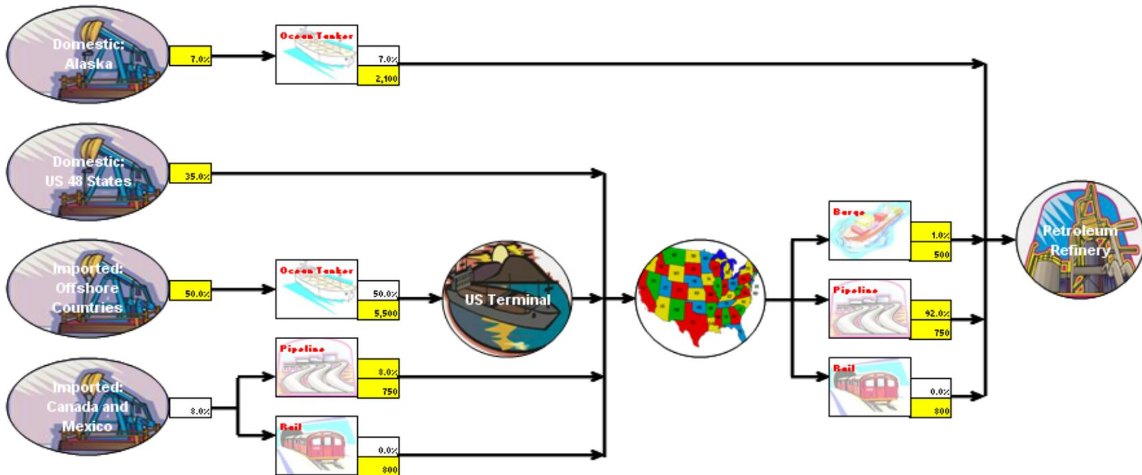
Figure 3.4.1 Transportation & distribution process diagram for conventional crude oil for use in U.S. refineries
