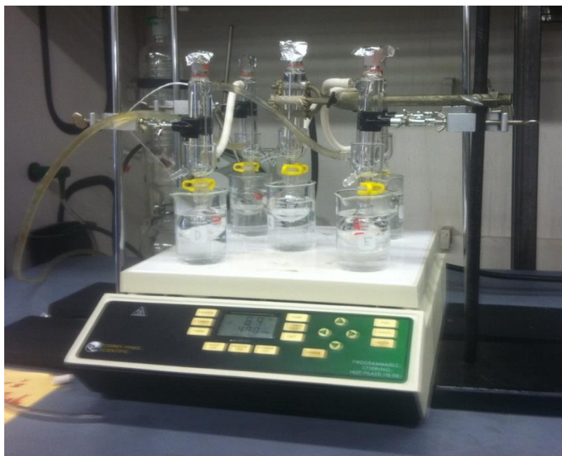
Figure 14: Reflux reactor experimental setup.
