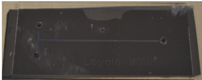
Figure 9: Straight microreactor with 3 cm nominal length.
