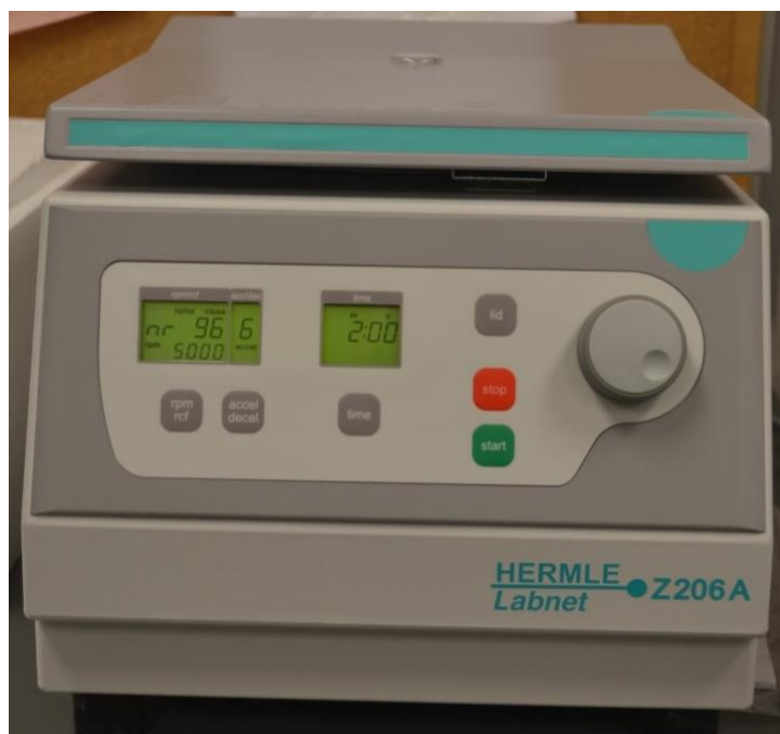
Figure 13: Hermle Z206A centrifuge.
