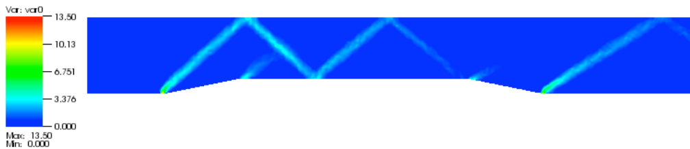
Figure 5.8 Magnitude of gradients in Mach number before range restraint
