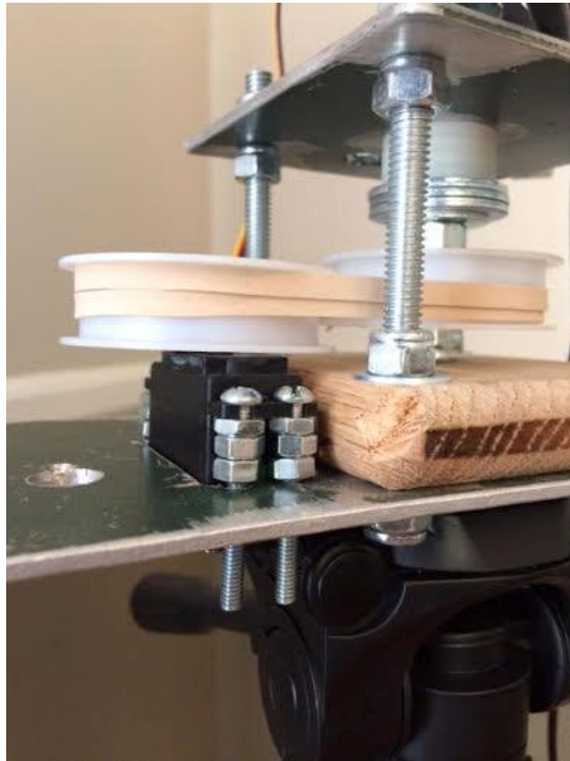
Figure 18: Complete Setup of X-Y Servo
