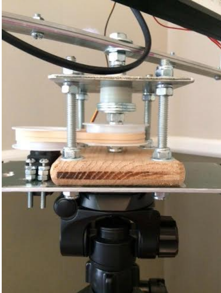
Figure 9: Active Tracker Base Attached to Tripod with View of X-Y Servo
