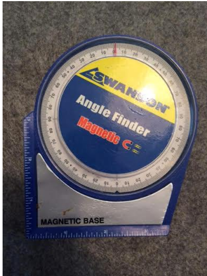
Figure 17: Swanson Inclinator Used for Testing
