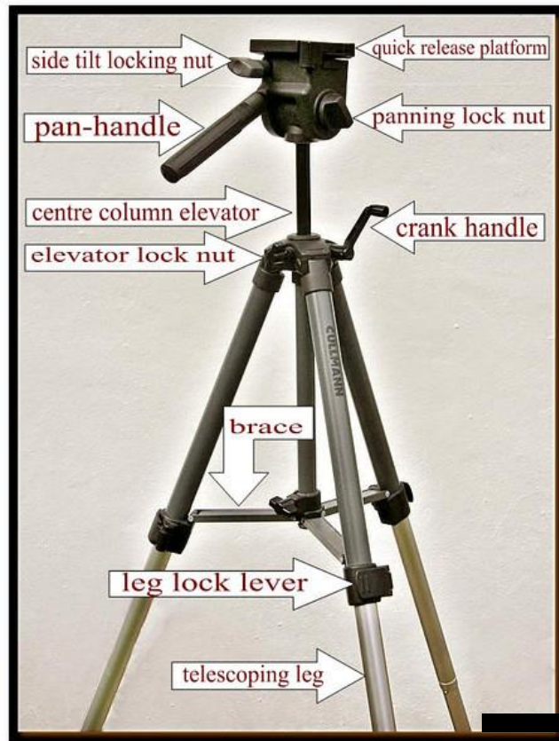
Figure 15: Tripod with part descriptions
