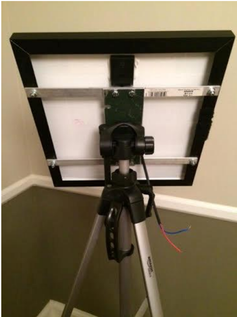
Figure 5: Rearview of the Manual Array Attached to the Tripod
