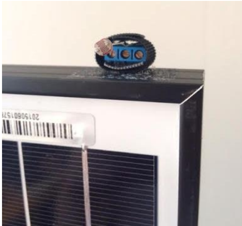
Figure 13: Placement of Light Dependent Resistor
