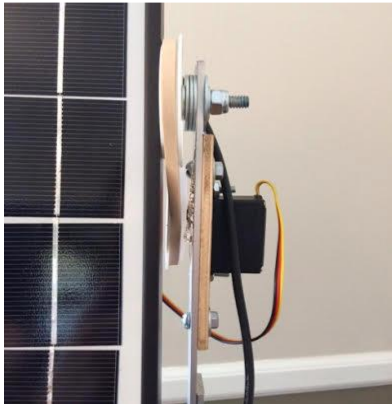
Figure 11: X-Z Plane Servo for the Active Tracker
