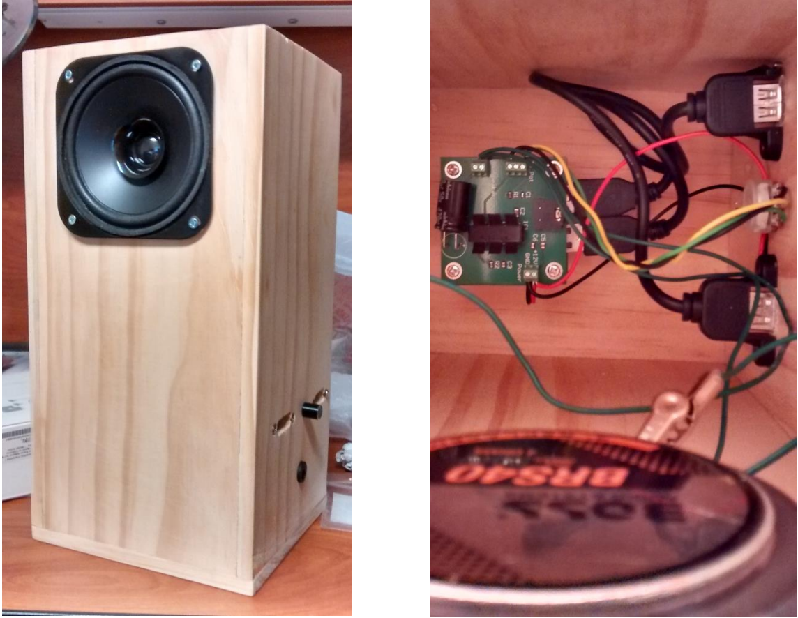
Figure 17 – Receiver base station prototype (left) Top-down view of receiver electronics (right)
