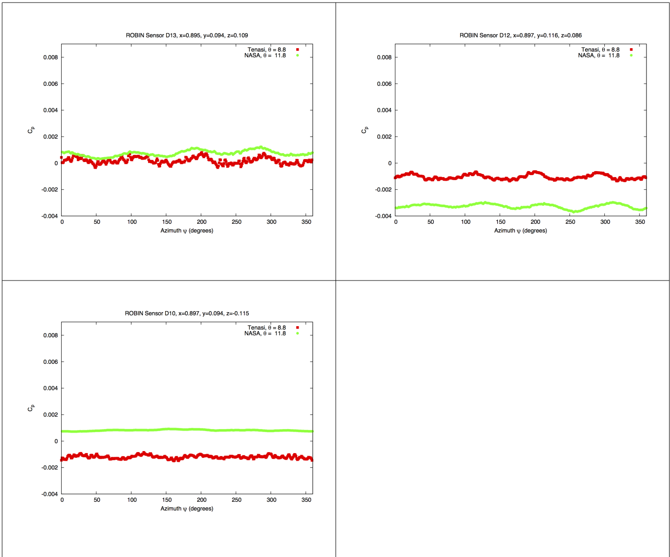
Figure 73 Pressure coefficient vs. rotor azimuth, sensors D13, D12, D10
