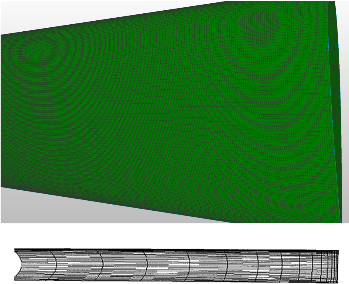
Figure 22 Tenasi isolated rotor blade surface mesh vs. TURBO blade surface mesh
