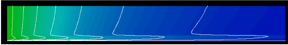
Figure 5.8 Contour plot of turbulent kinetic energy for neutral ABL
