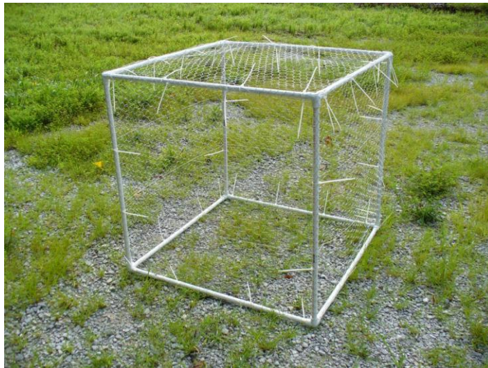
Figure 2.3 Example herbivory study enclosure constructed of a PVC pipe frame enclosed with wire mesh secured by cable ties.
