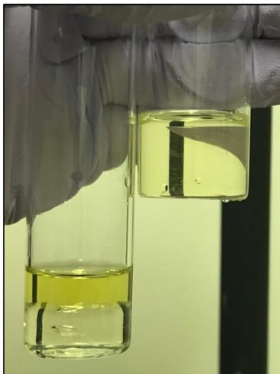
**Figure 32.** Micro/millifluidic device biodiesel production experiment products (left) and pure vegetable oil (right).
