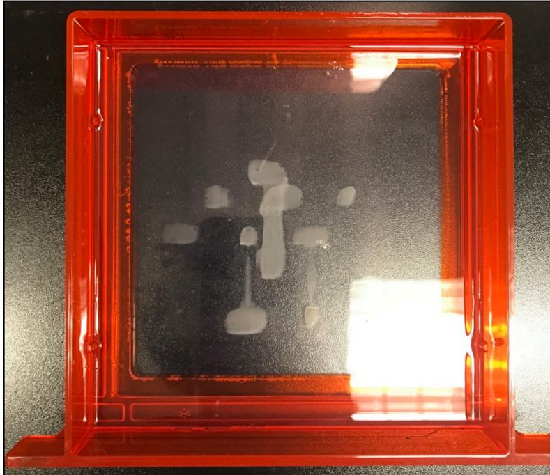
**Figure 5.** Clouding in resin tank after repeated use.
