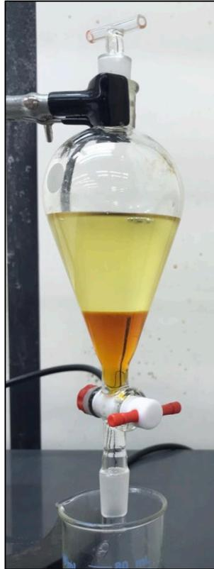
**Figure 30.** Batch biodiesel experiment products before separation. Biodiesel is the top layer, while the bottom layer is mainly glycerin.
