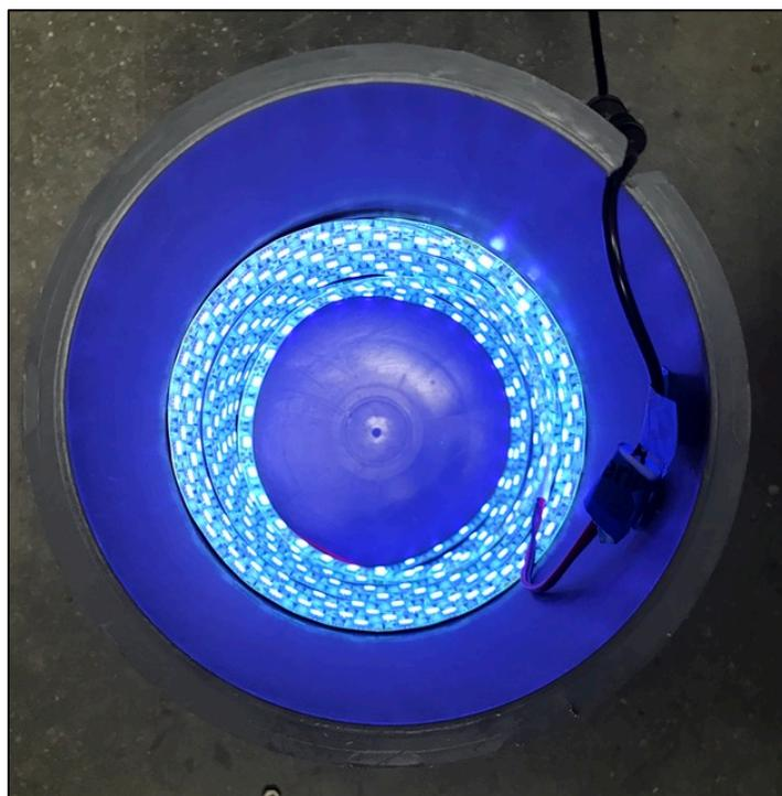
**Figure 4.** Post-cure chamber without cover.
