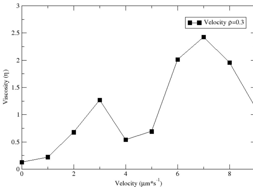
The explanation for the two velocities in which the system experiences shear thinning is that at  $3 \mu\text{m}^*\text{s}^{-1}$ , a large cluster just split into two smaller clusters. As velocity increases, the two smaller clusters begin to increase in size resulting in two large dynamic clusters interacting with each other. This leads to a phase separation of a few highly dense clusters surrounded by a dilute gas phase.
