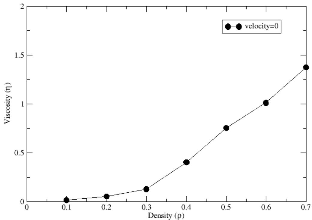
The explanation for the dramatic increase in viscosity once density hits 0.4 is that the clusters begin to split apart, but then those clusters increase in size through time resulting in a phase separation.
