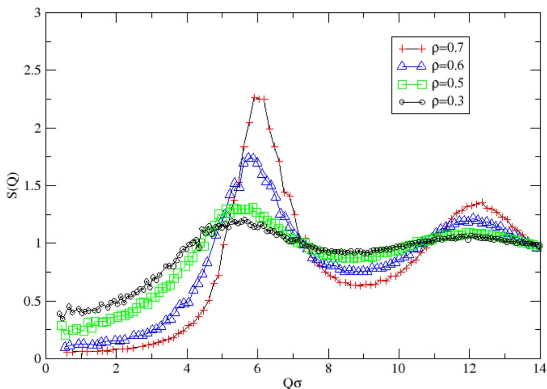
With velocity set to  $0 \mu\text{m} \cdot \text{s}^{-1}$ , the intensity of the scattering light ( $Q$ ) has to be relatively high ( $6 \sigma$ ). With the particles being passive Brownian particles, the low-density colloids have a lower probability of interacting with each other as opposed to the high-density colloids.
