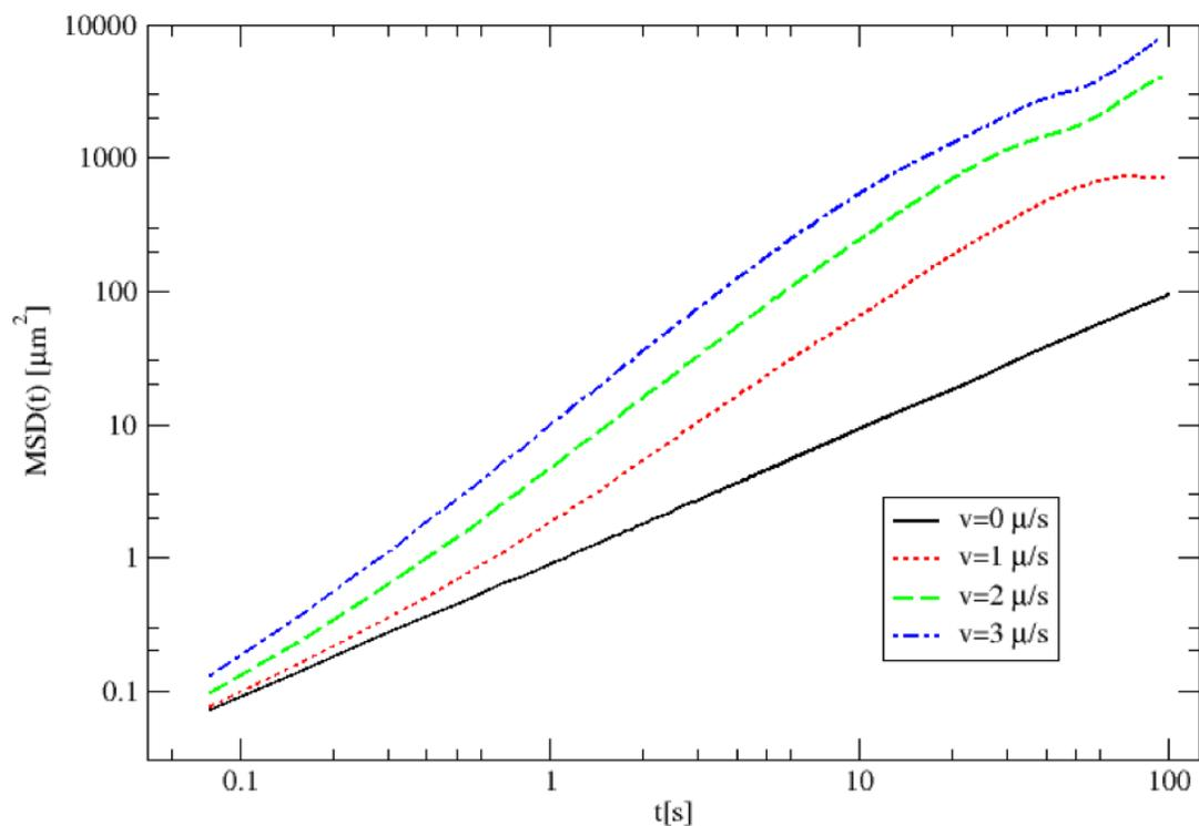
Behavior is as expected and opposite from collective motion solutions. The lowest velocity contains particles that stay closer together and do not move far, whereas the highest velocity contains particles that are more spread out and travel farther.
