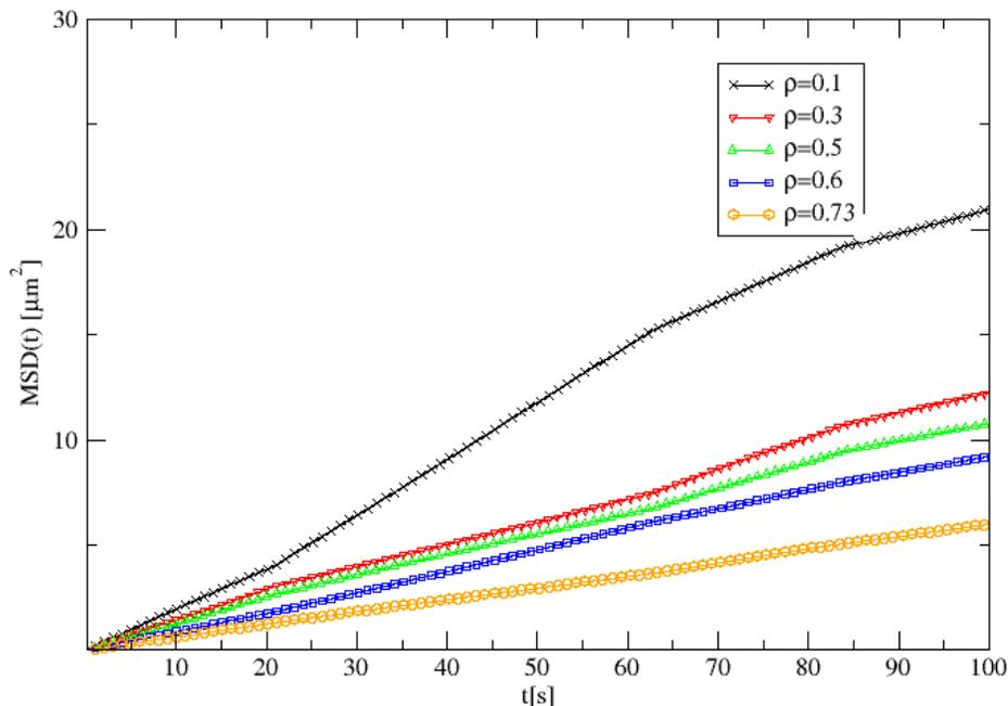
As mentioned for Figure 3.1.1, the results for collective motion are opposite for the distance travelled. In this instance, the varying densities are described. The lower densities do not interact with each other as much as the higher densities which allow for a higher distance travelled for lower density systems.
