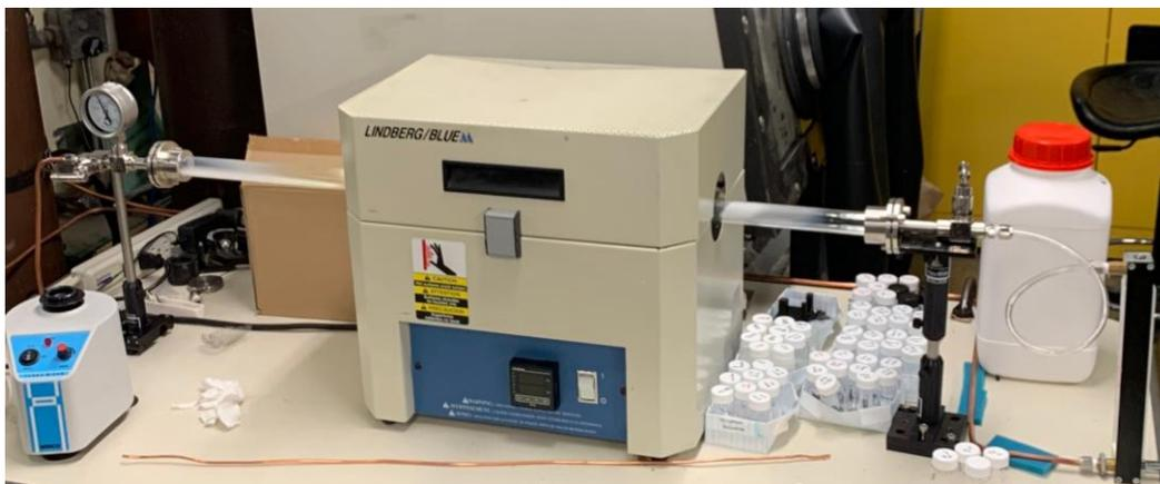
**Figure 2** Lindberg/Blue Mini-Mite Tube Furnace and piping setup
