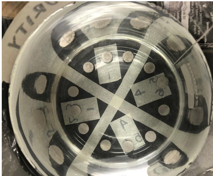
Figure [2]: Sample layout of coupons in immersion testing beaker.
