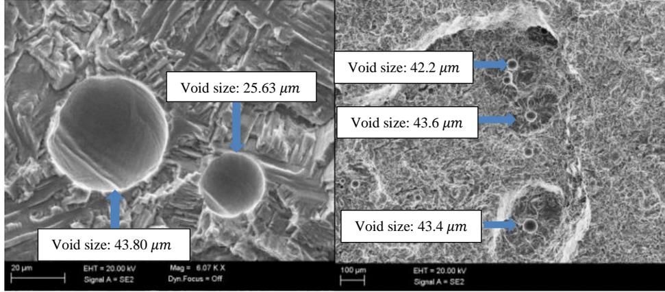
Figure 1- Void formation in Ti-6Al-4V fabricated using LENS method (These features were quantified for MSF model).
