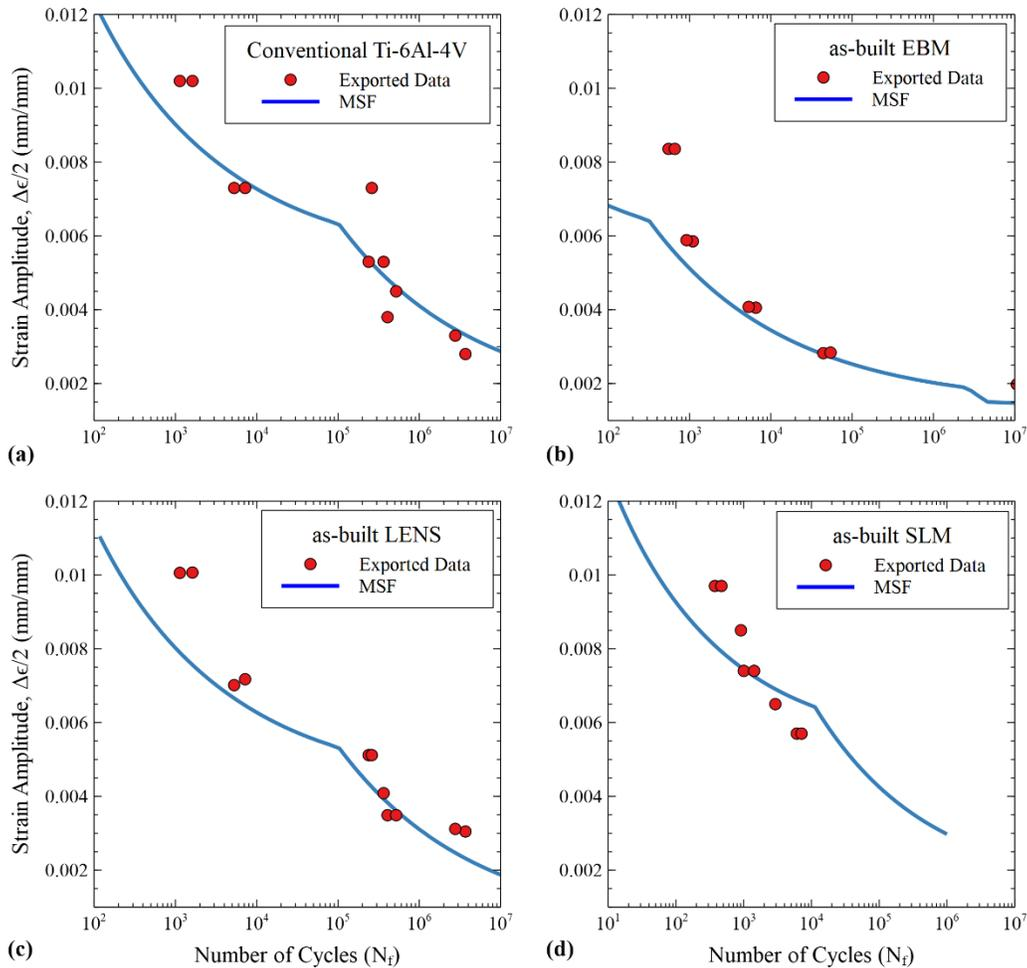
Figure 2- Calibrated fatigue curves using the multistage fatigue model for (a) conventional Ti-6Al-4V, (b) as-built EBM, (c) as-built LENS, and (d) as-built SLM.
