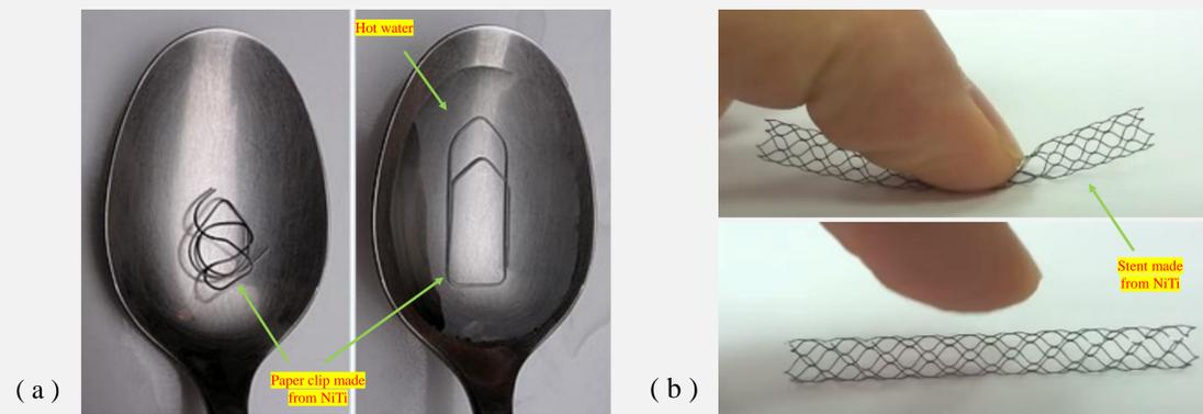
Fig. 1 – a) Shape memory effect in NiTi: Deformed paper clip recovers its original shape in the hot water. b) Superelasticity in NiTi: Reversible elastic behavior helps inserted collapsed stent in the artery to expand to its original shape.
