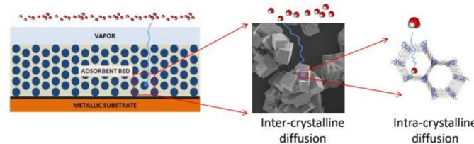
Figure 1: (left) Vapor capture by adsorbent bed with heat sink substrate. (center) Macroporosities characterize vapor diffusion and are temperature dependent. (right) Microporosities characterizes saturation limitations with rate limited temperature dependence.
