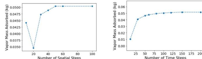
Figure 6: Convergence Studies (left) Spatial Convergence: the mesh adequately resolved at  $nx = 50$ .  $nx = 60$  was used for subsequent investigation. (right) Temporal Convergence: the time stepping adequately resolved at  $nt = 125$ .  $nt = 150$  was used for subsequent investigation.
