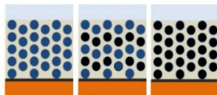
Figure 4: Each iteration of the ANN optimization increases the distribution of the Phase Change Material beads (black) replacing Adsorbent beads (blue). The results of such iterations are displayed to the right.
