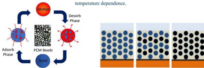
Figure 3: Phase Change Material Cycle, During the Adsorb phase the PCM captures heat and during the Desorb phase the PCM releases heat.
