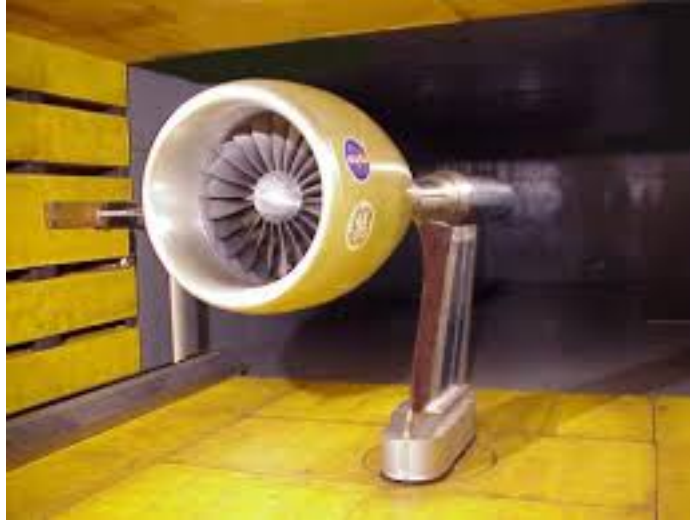
Figure 3.1 SDT2-R4 installed in wind tunnel.
