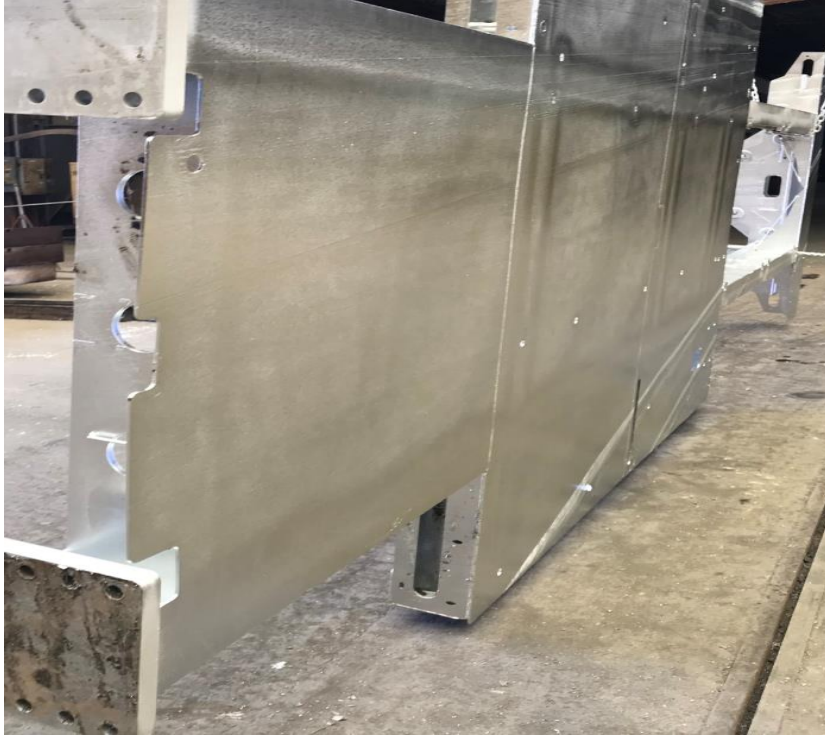
Figure 3.12 New design post hot-dip galvanizing (shared with permission from Valmont)
