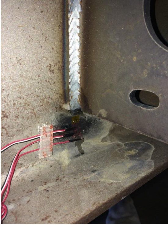
Figure C1.6 Sample strain gauge placement at weld toe
