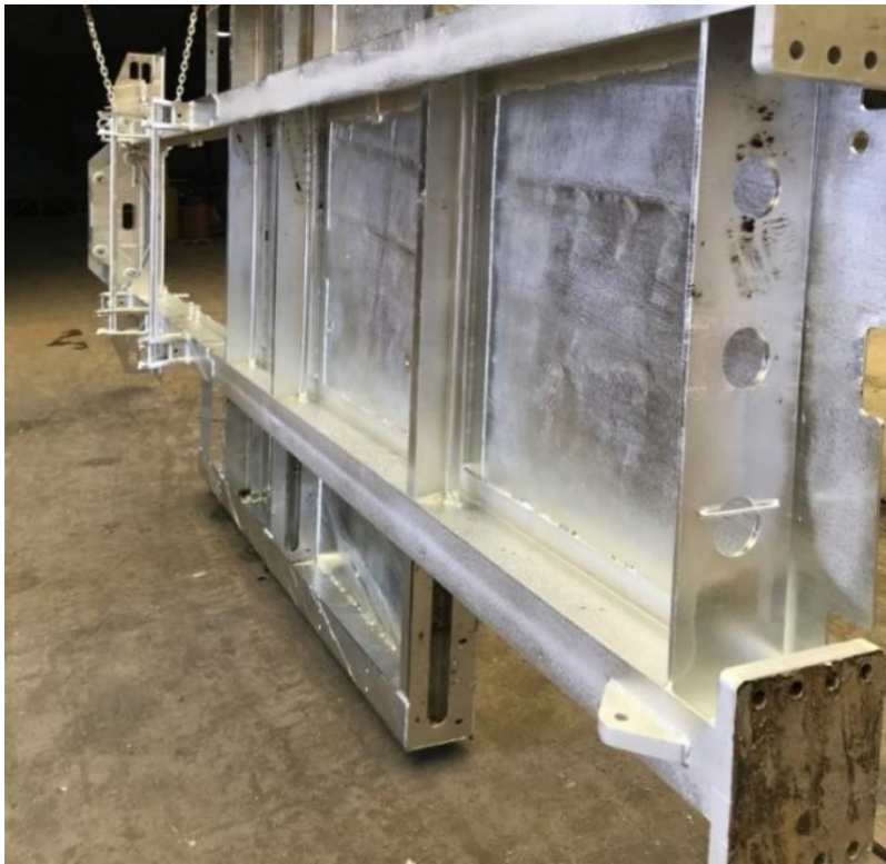
Figure 3.11 New design post hot-dip galvanizing (shared with permission from Valmont)
