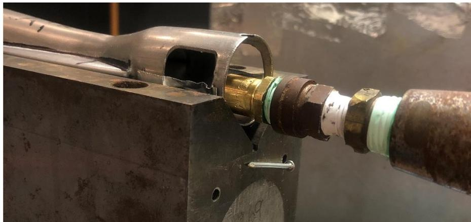
Figure 3.6 Orifice Adjustment for Off-Center
