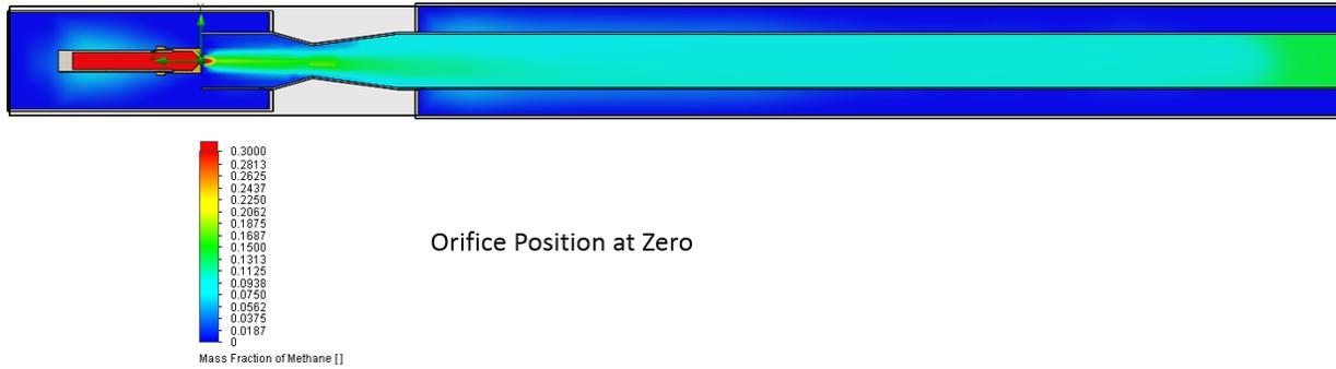
Figure 4.9 Cut-Plot, Computer Model with Orifice Depth at Zero
