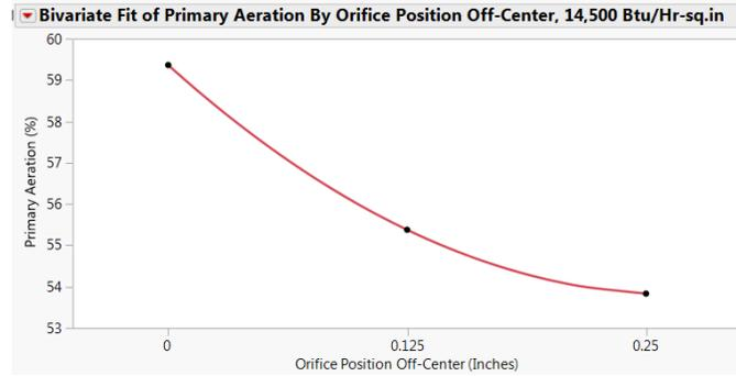
Figure 4.1 Orifice Position Off-Center vs. Primary Aeration
