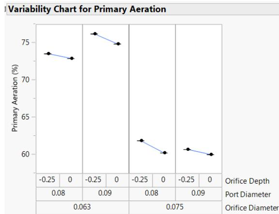
Figure 4.6 Variability Chart, Level Settings vs. Primary Aeration, Lab Experiment 3
