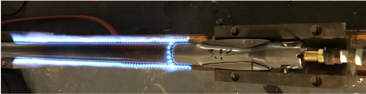
Figure 3.4 Fired Burner on Test Bench
