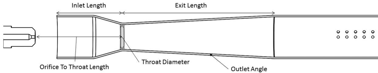
Figure 2.4 Venturi Geometry
