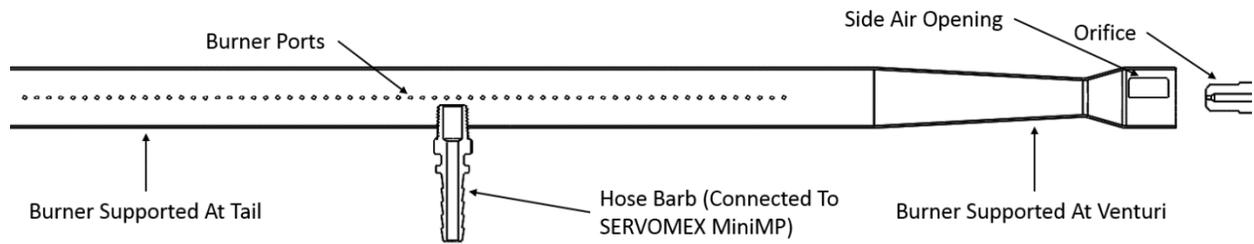
Figure 3.3 Experiment Testing Oxygen Tapping
