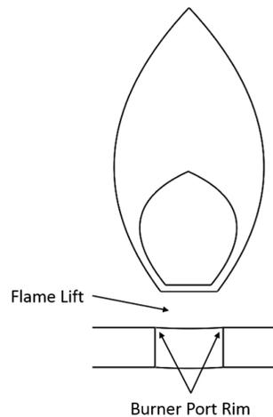
Figure 2.8 Flame Lift Example
