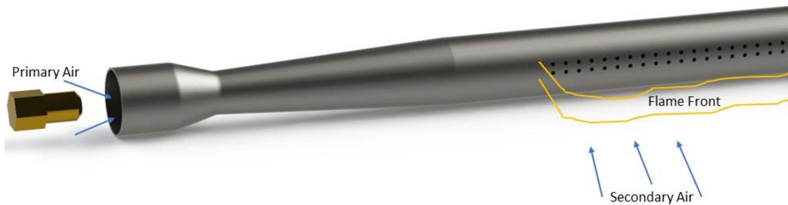
Figure 2.2 Primary and Secondary Aeration Visual Explanation
