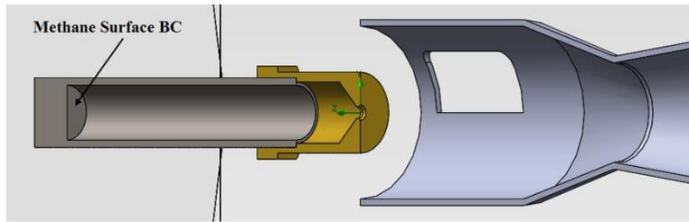
Figure 3.12 Flow Simulation Gas Inlet Boundary Condition
