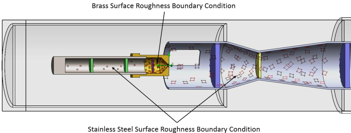
Figure 3.13 Inlet Boundary Conditions
