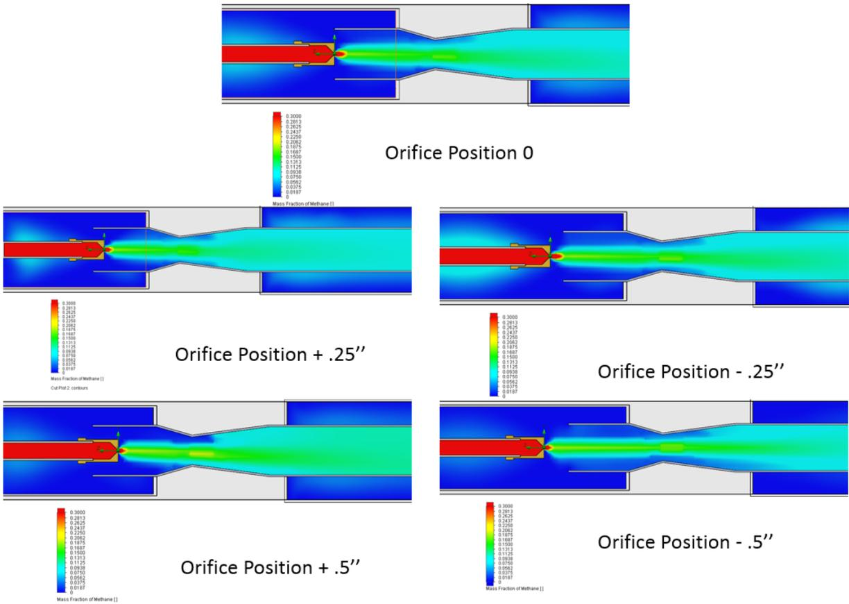
Figure 4.10 Cut-Plot, Computer Model at Venturi for all Depths
