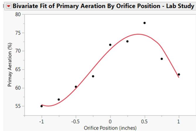
Figure 4.2 Orifice Position Depth vs. Primary Aeration
