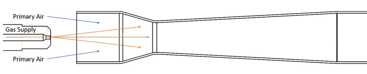
Figure 2.1 Primary Aeration and Gas Supply at Burner Inlet
