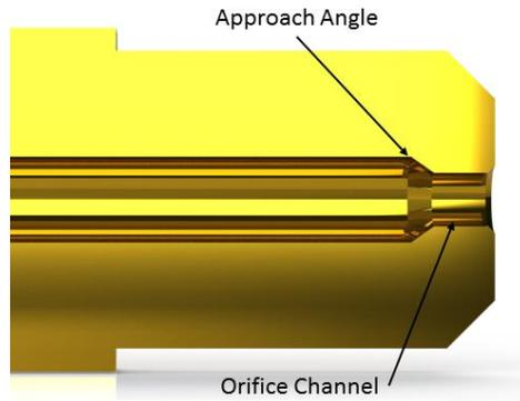
Figure 2.3 Orifice Internal Geometry
