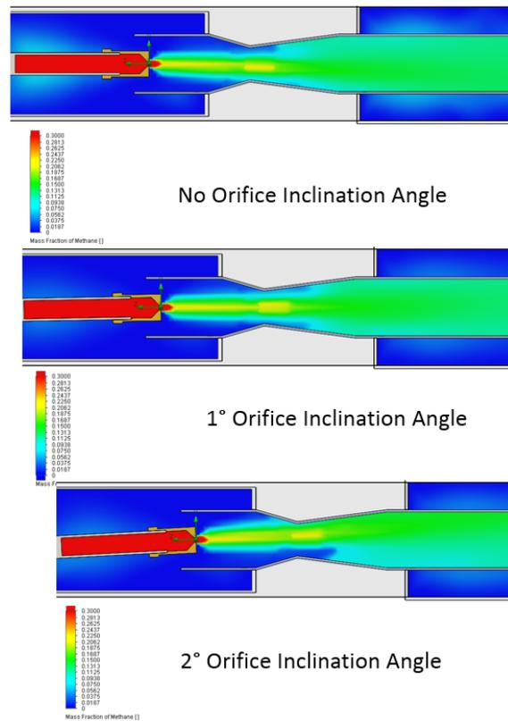
Figure 4.11 Cut-Plot, Computer Model Orifice Inclination Angle Study
