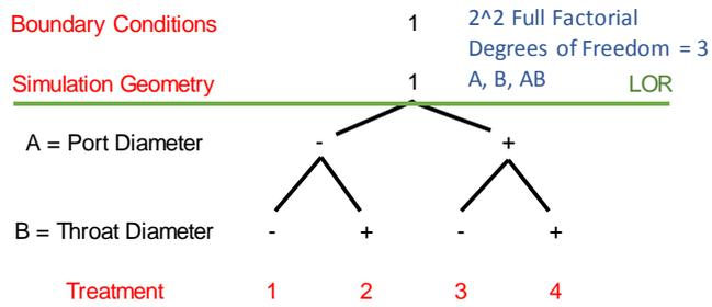
Figure 3.18 Factor Relationship Diagram Computer Modeling DOE
