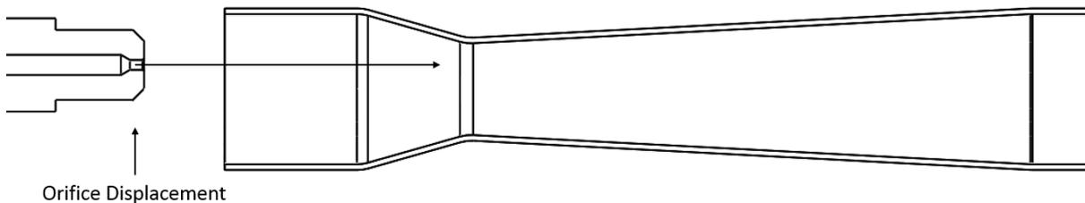
Figure 2.6 Orifice Displacement from Center of Burner
