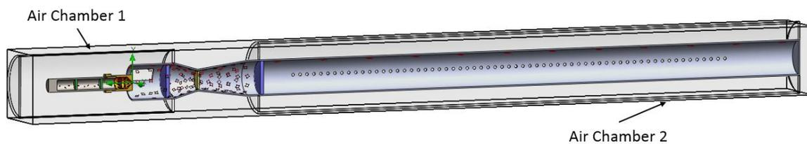
Figure 3.11 Flow Simulation Set-Up
