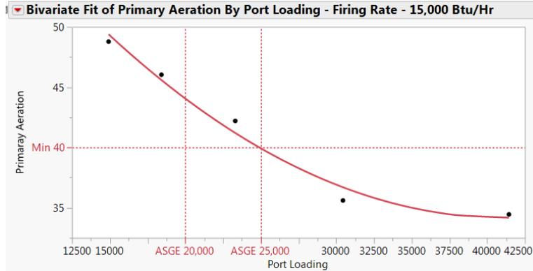
Figure 4.13 Computer Simulation, Port Loading vs. Primary Aeration
