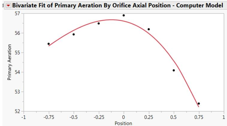
Figure 4.8 Computer Model, Orifice Depth vs. Primary Aeration
