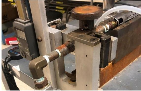
Figure 3.5 Test Bench Height Adjustment
