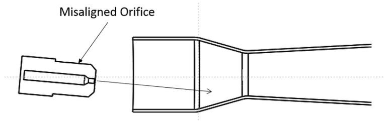
Figure 2.5 Orifice Misalignment from Centerline of Burner
