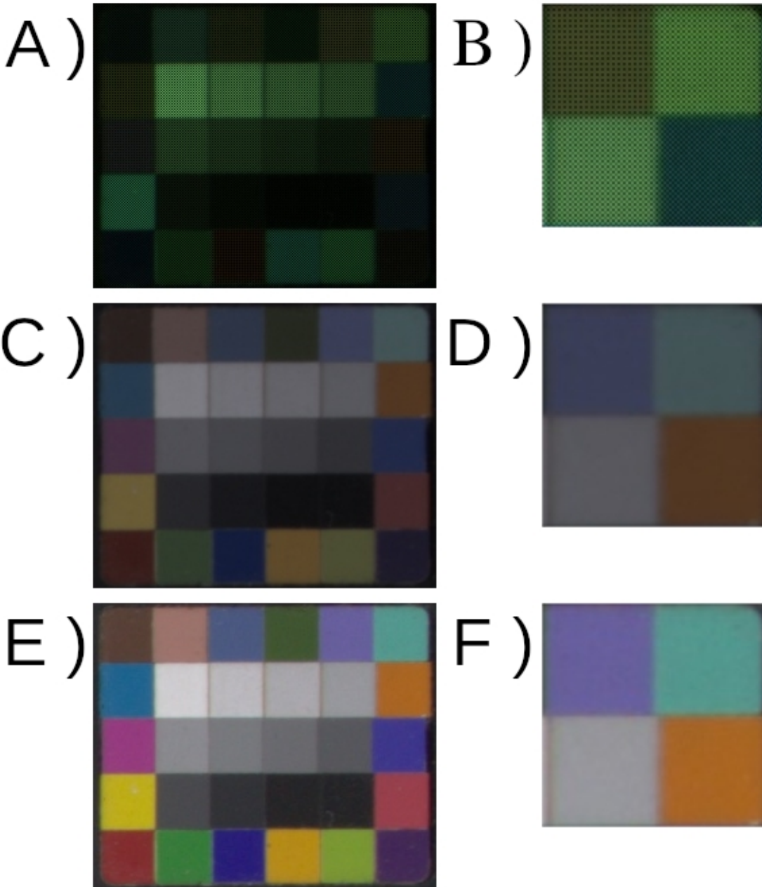
A color reference chart from a herbarium specimen image at varying states of processing. Subfig "A" shows a RAW image's bayer pattern before demosaicing. Subfig "B" is a portion of "A" zoomed to 200%. Subfig "C" has been demosaiced using a linear algorithm and given equal white balance weights. Subfig "D" is a portion of "C" zoomed to 200%. Both "C" and "D" are indicative of demosaic settings used in phase one of HerbASAP image processing. Subfig "E" has been demosaiced using the adaptive homogeneity-directed demosaicing algorithm with white balance weights calculated from subfig "C". Subfig "F" is a portion of "E" zoomed to 200%. Both "E" and "F" are indicative of demosaic settings used in phase two of image processing in HerbASAP.
