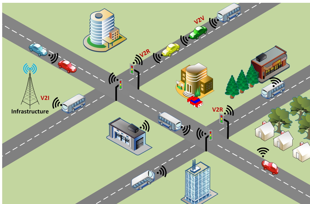
Figure 2.1 Smart city demonstrating how various devices are able to communicate through, vehicle-to-vehicle, vehicle-to-RSU, and vehicle-to-infrastructure to aid in efficient operations of the city
