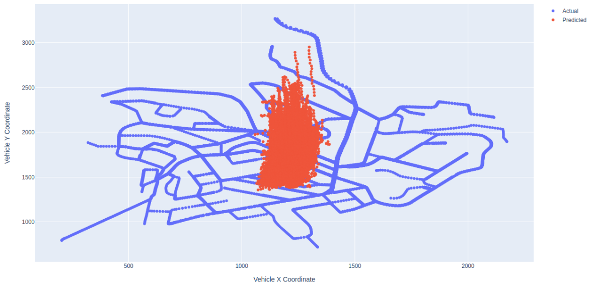
Figure 6.9 BIRCH Actual vs Predicted for LinearRegression. Our data points are centered because LinearRegression tries to create a “Best Fit” for all data points
