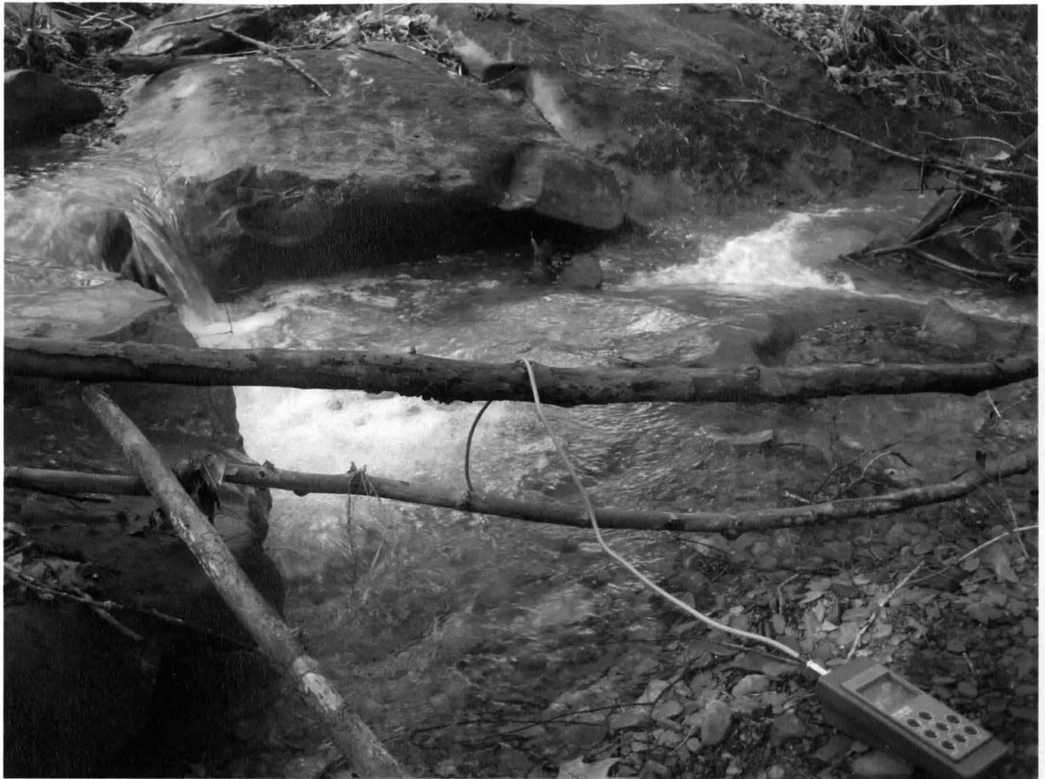
Figure 3. The Hanna pH & temperature meter used in this research tests the waters of Mikel Branch, a stream with orange staining on the rocks that is indicative of the impacts of Acid Mine Drainage. The meter is in the bottom right of the photo.
