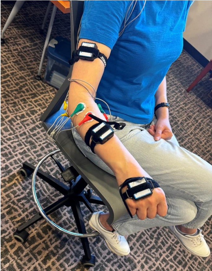
Figure 4.4 IMU sensors and EMG sensors placements for recording data
