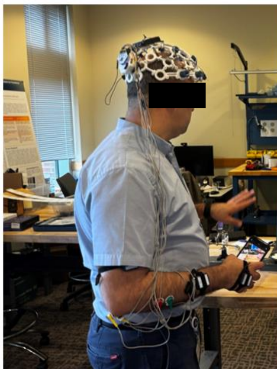
Figure 4.7 Placement of EEG, EMG, and IMU sensors for collecting data from participant
