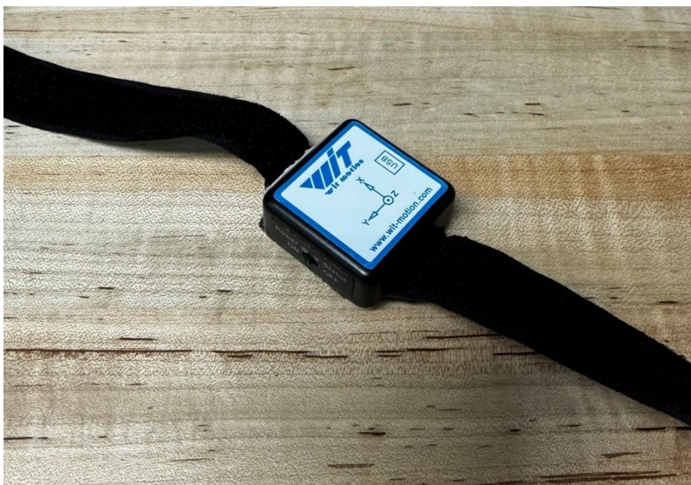
Figure 3.4 IMU device is used to record data in three dimensions: X, Y, and Z
